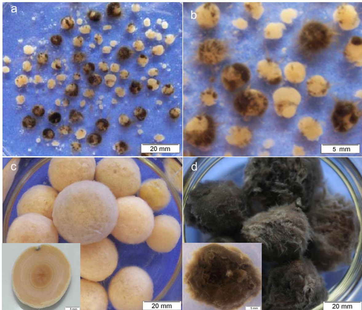
Fig. 1. Photographs of the aerobic granular sludge in the two batch reactors: (a) and (b) seed granules from a SBR and (c) large bacterial granules from R1 and (d) large fungal granules from R2, respectively, after 120 days of cultivation.
