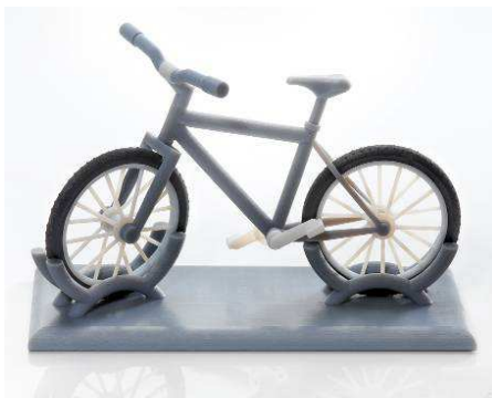
Fig. 2. A multi-material bicycle prototype fabricated by Connex500™ multi-material 3D printing system (Object, 2011b)
