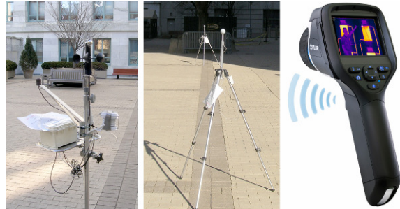
Figure 6, Measurement Devices in use including 38mm Greyball Thermometer, portable weather station, and infrared camera.
