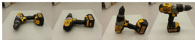
Fig. 2. All four stable pose classes for a gun-type drill.
