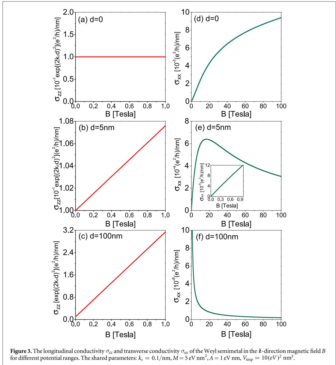
**Figure 3.** The longitudinal conductivity  $\sigma_{zz}$  and transverse conductivity  $\sigma_{xx}$  of the Weyl semimetal in the  $\hat{z}$ -direction magnetic field  $B$  for different potential ranges. The shared parameters:  $k_c = 0.1/\text{nm}$ ,  $M = 5 \text{ eV nm}^2$ ,  $A = 1 \text{ eV nm}$ ,  $V_{\text{imp}} = 10(\text{eV})^2 \text{ nm}^3$ .
