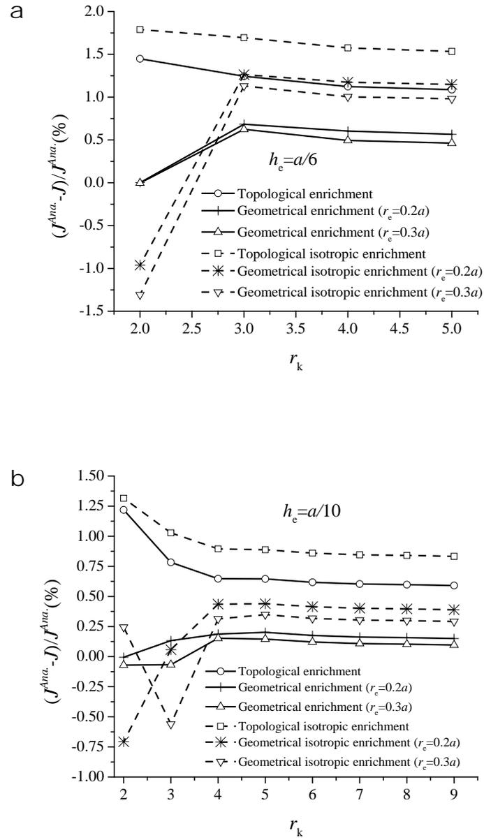
Figure 4. Domain independence study for interface crack: (a)  $h_e = a/6$ ; (b)  $h_e = a/10$ .
