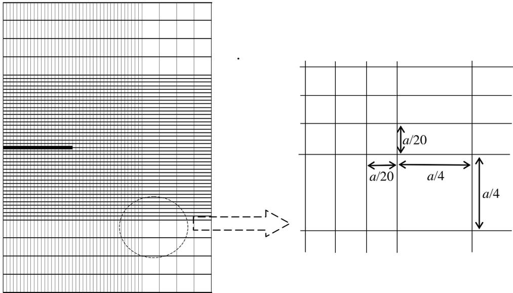
Figure 6. The non-uniform mesh with local refinement in the vicinity of the crack:
