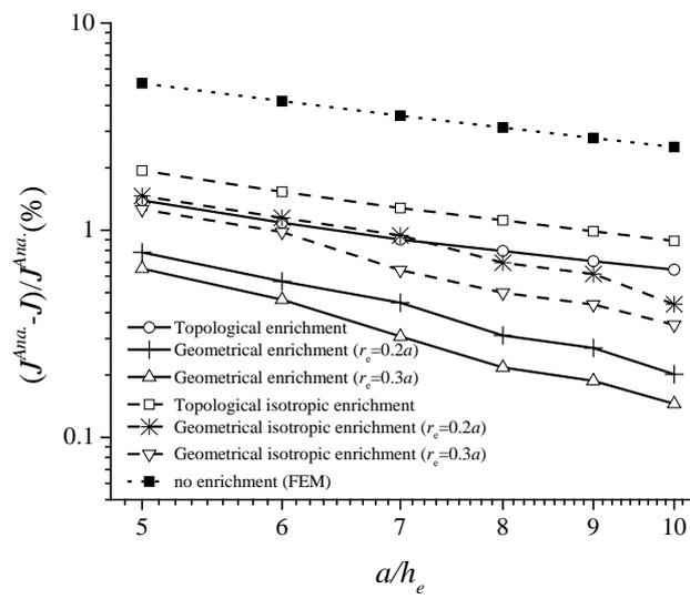
Figure 5. Convergency study of the  $J$ -integral with respect to mesh density for interface crack.
