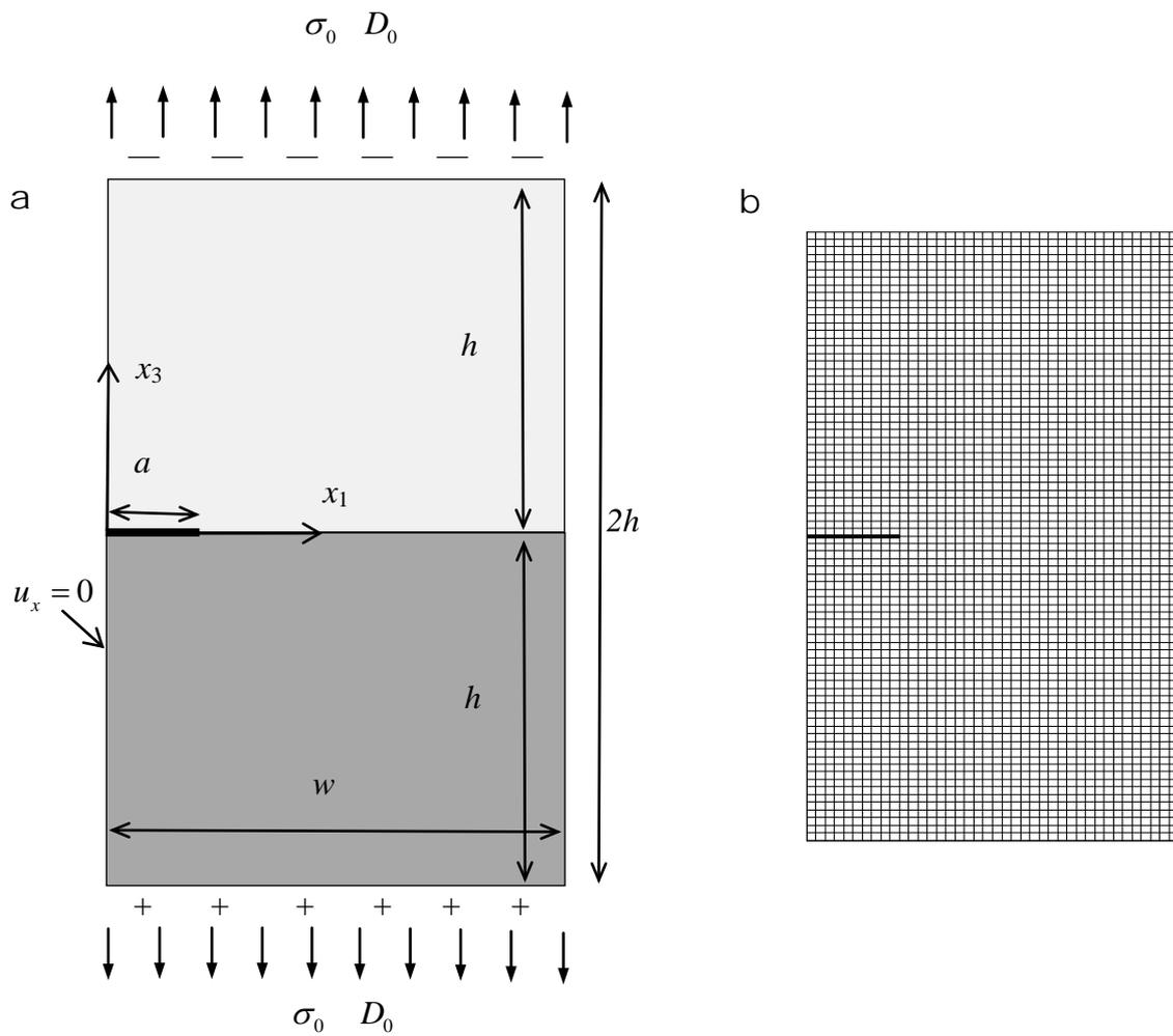
Figure 3. Interface crack under electromechanical load (half -model): (a) problem configuration; (b) uniform mesh in the vicinity of the crack ( $h_e = a/10$ ).
