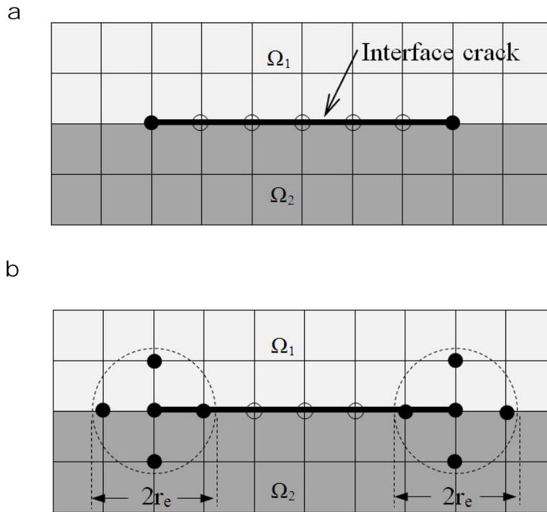
Figure 2. Enriched nodes for a bimaterial interface crack: (a) topological enrichment; (b) geometrical enrichment (the nodes enriched by the Heaviside function are marked with open circles whereas the nodes enriched by crack-tip enrichment functions are marked with filled circles).
