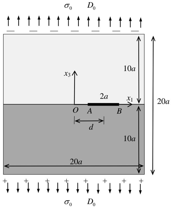
Figure 7. An interface crack between two finite piezoelectric plates.
