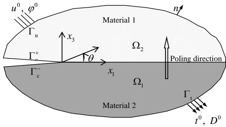
Figure 1. An interface crack in a piezoelectric bimaterial.
