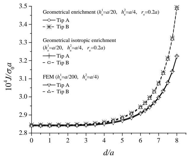
Figure 8. Normalized  $J$ -integral with respect to the location of interface crack.
