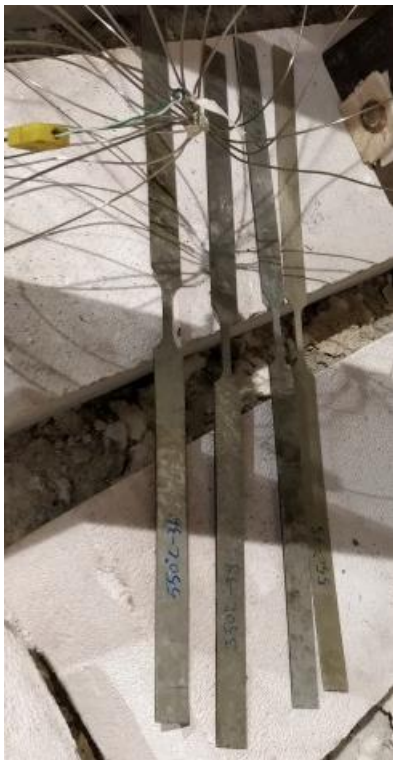
Figure 2: Coupon specimens heated in LPG furnace (left) and in electric furnace (right)
