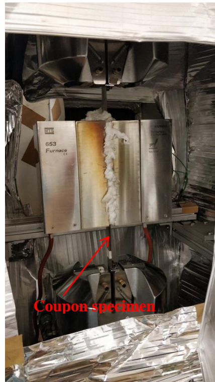
Figure 2: Coupon specimens heated in LPG furnace (left) and in electric furnace (right)
