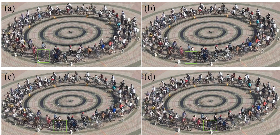
Fig. 6. Photographs of following behavior in the 90-bicycle experiment. The focal cyclist (green box) followed those ahead.
