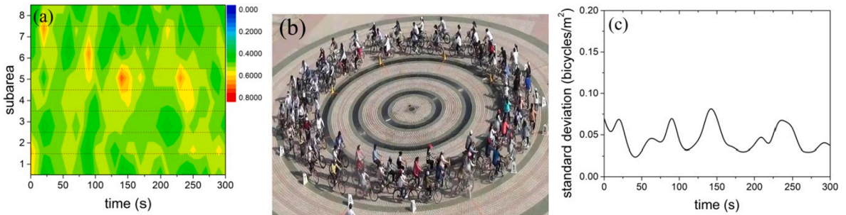
Fig. 17. Results of a 90-participant experimental run: (a) density evolution in the eight subareas, unit: bicycles/m 2 ; (b) snapshot photograph; (c) standard deviation of bicycle density in the eight subareas. Dashed lines represent subarea boundaries.
