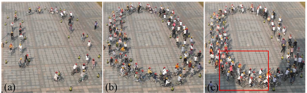
Fig. 22. Snapshot photograph on the playground-like track: (a) 30 participants; (b) 90 participants; (c) 100 participants. The red box shows a jam area.
