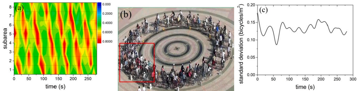
Fig. 20. Results of the 100-participant experimental run: (a) density evolution in the eight subareas; (b) snapshot photograph; (c) standard deviation of bicycle density in the eight subareas as a function of time. Dashed lines represent subarea boundaries and the red box represents the jam area.
