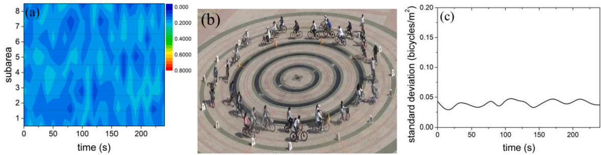
Fig. 19. Results of the 30-participant experimental run: (a) density evolution in the eight subareas; (b) snapshot photograph; (c) standard deviation of bicycle density in the eight subareas. Dashed lines represent subarea boundaries.
