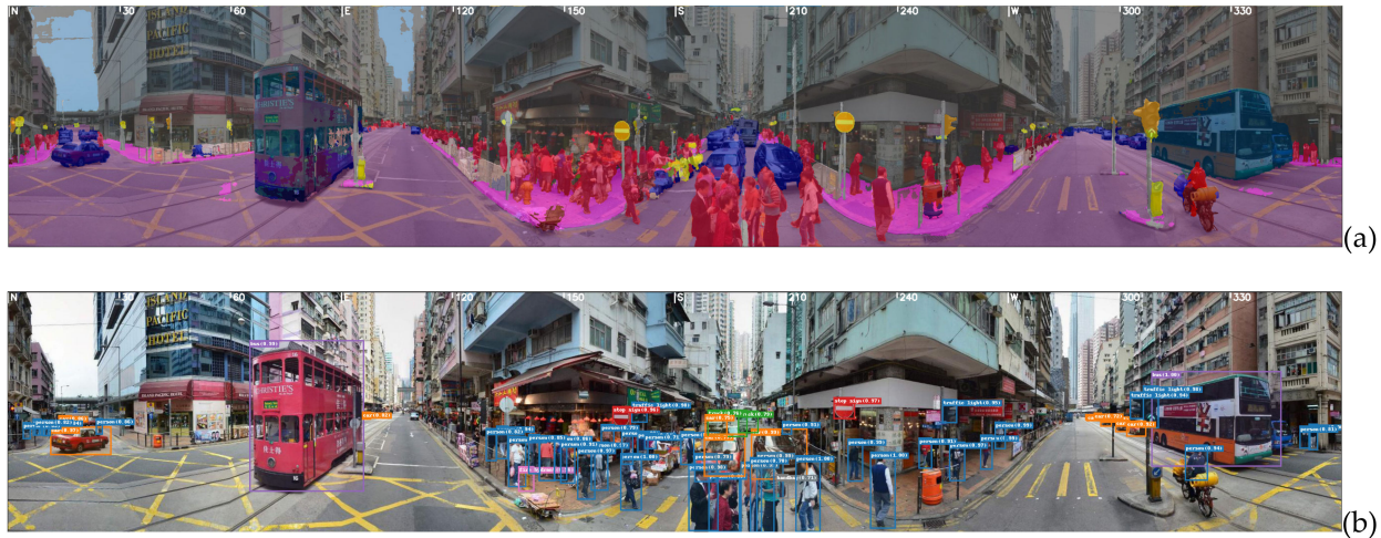
Figure 7. Results of semantic segmentation and object recognition. (a) Example of semantic segmentation, color indicates class; (b) example of object recognition, color of a bounding box indicates class.
