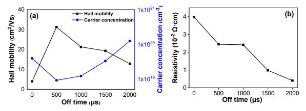
**Figure 6.** Electrical properties of ITZO films deposited at different pulse off-times: (**a**) the carrier mobility and carrier concentration and (**b**) the films' resistivity.
