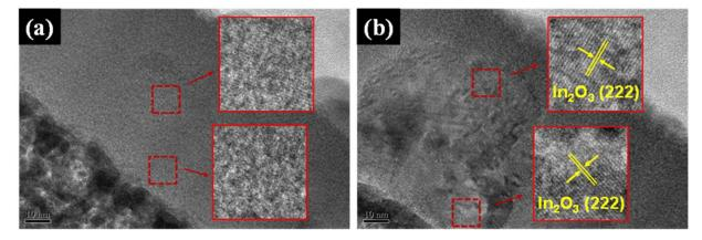
**Figure 4.** The cross-sectional TEM images as well as the corresponding enlarged images of ITZO films deposited with pulse off-times of (**a**)  $0 \ \mu$ s and (**b**) 2000  $\mu$ s.
