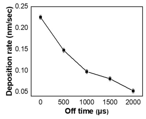
Figure 2. Deposition rate at different pulse off-times.
