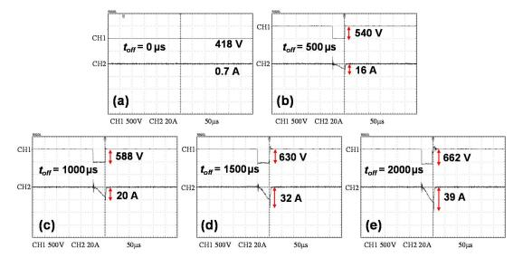
**Figure 1.** The sputtering voltage and current with different sputtering pulse off-times ( $t_{off}$ ): (**a**) 0 µs, (**b**) 500 µs, (**c**) 1000 µs, (**d**) 1500 µs, and (**e**) 2000 µs.
