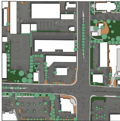
Fig. 4. Same plan view as in Fig. 3, but after application of each mitigation strategy that comprises the “combined” strategy in Fig. 3, including increased: rooftop albedos (left; white areas), solar panel and sail cloth shading (middle; grey and pink areas, respectively), and vegetative greening (right). See text for explanation of each strategy. (For interpretation of the references to color in this figure legend, the reader is referred to the Web version of this article.)
