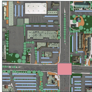
Fig. 4. Same plan view as in Fig. 3, but after application of each mitigation strategy that comprises the “combined” strategy in Fig. 3, including increased: rooftop albedos (left; white areas), solar panel and sail cloth shading (middle; grey and pink areas, respectively), and vegetative greening (right). See text for explanation of each strategy. (For interpretation of the references to color in this figure legend, the reader is referred to the Web version of this article.)
