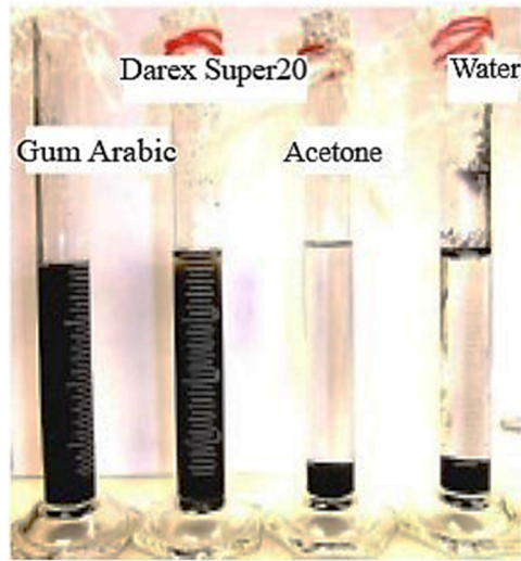
Figure 3: Ultrasound combined with Darex Super20 dispersion effect [41].
