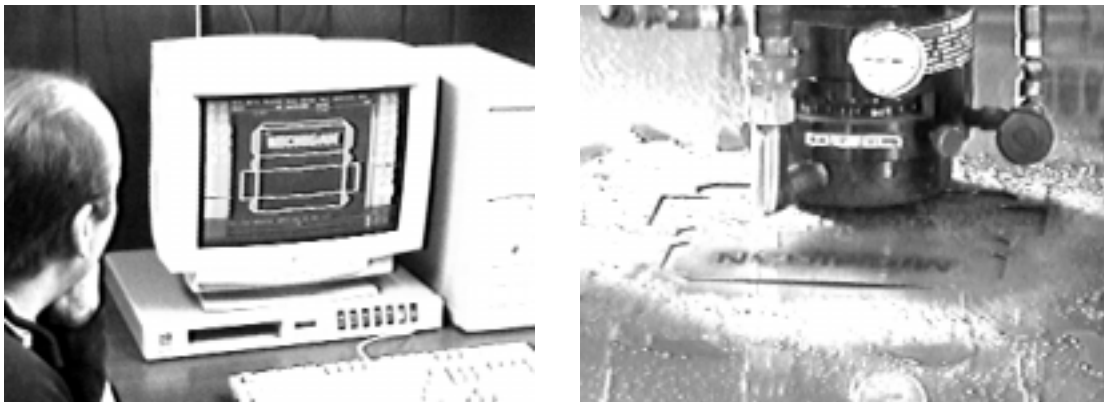
Figure 38: Manufacturer's computer & numerical controlled laser cutter
