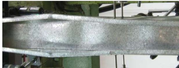
Figure 7: Experimental evidence of the occurrence of local/distortional interaction (specimen T1.5-HSS-1)
