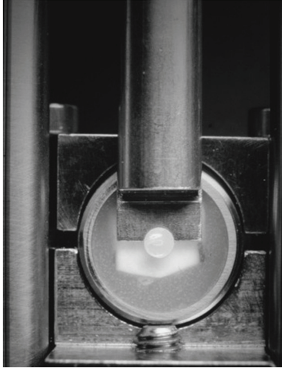
FIGURE 2: The specimen in the shear bond strength test.
