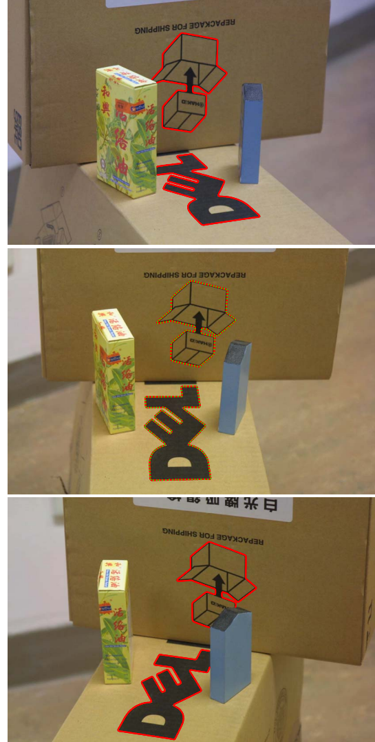
Figure 2. The sequence of images. The extracted curves are shown in red. The curves in the second image are selected as reference curves and the green dots are the representative points.
