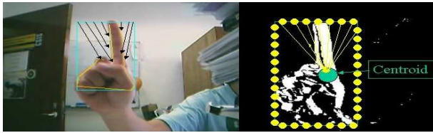
Fig. 5. The left image is the input image. The right image shows the potential region in white color. The arrow shows the searching path. By searching along the line joining the initial position and the centroid, the pixel with strong edge information is picked as potential contour.
