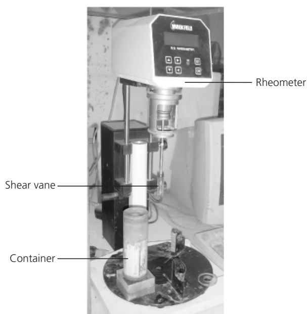
Figure 3. Rheometer, shear vane and container
