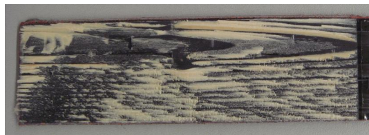
(a) Side A bonded FRP (Specimen 120A-2)
