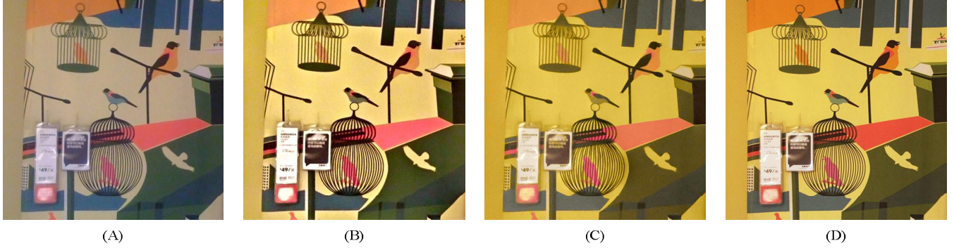
Figure 4: (A) is an original photo taken by iPhone 3G while (D) is the reference photo taken by Canon 5D Mark II. (B) is the result from an affine color mapping while (C) is the result from a quadratic color mapping. Between (B) and (C), (C) is overall visually closer to (D).
