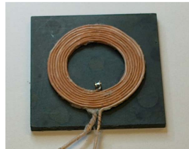
Fig. 16. Receiver winding and receiver ferrite plate.
