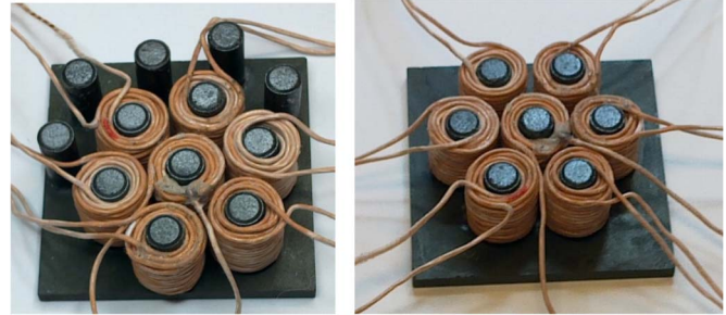
Fig. 15. (Left) Worst position and (right) best position winding arrays.
