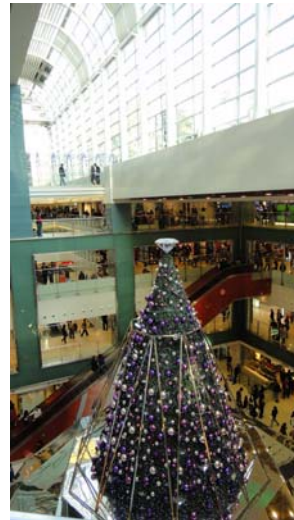
Fig. 1: High combustible content in a tall hall
