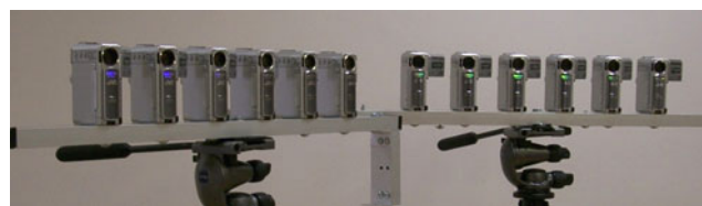
Figure 2 Plenoptic videos: Multiple linear camera array of 4D simplified dynamic light fields with viewpoints constrained along line segments. The camera arrays developed at [24]. Each consists of 6 JVC video cameras.
