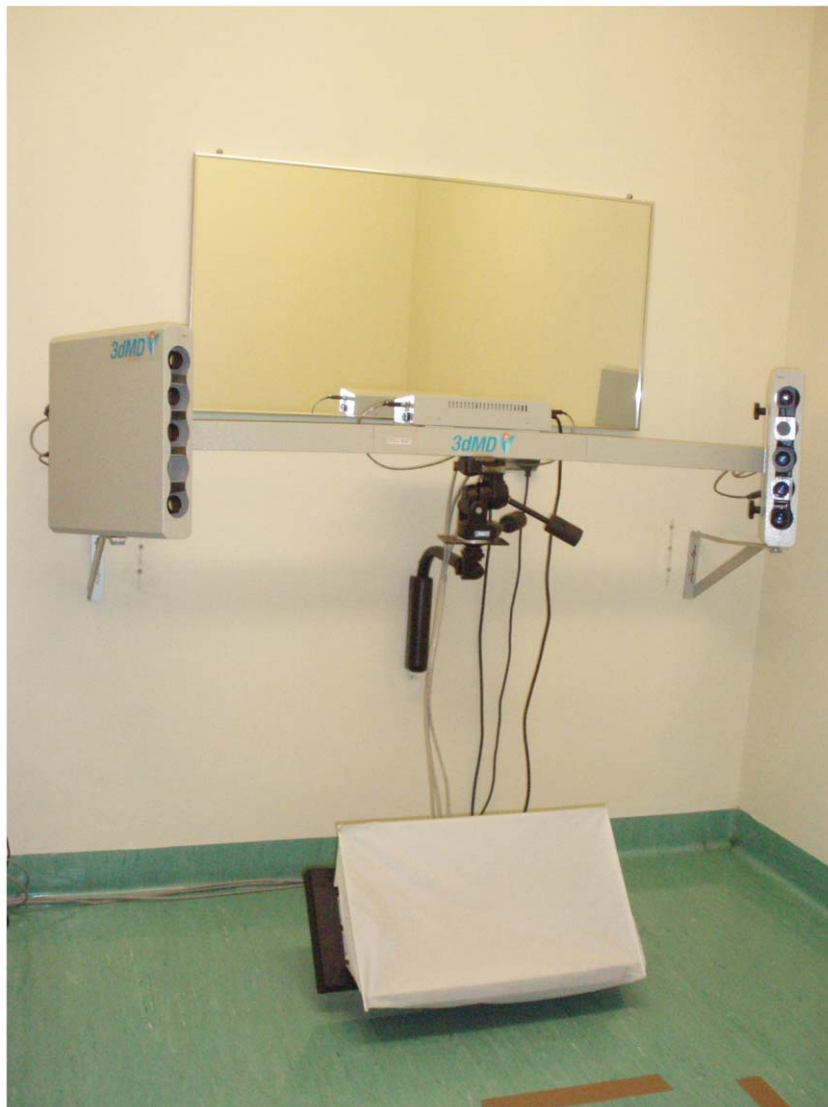
Figure 2. The 3dMDface stereophotographic system.
