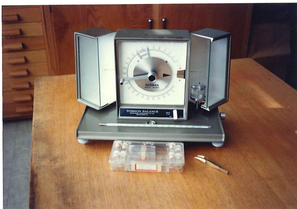
Plate 3.3 Berman torsion balance used for specific gravity determination of heavy mineral grains.
