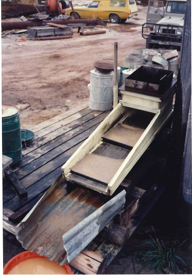
Plate 3.1 A short sluice box used for the concentration of heavy minerals.
