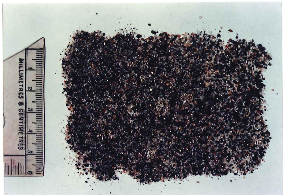
Plate 4.6 A typical heavy mineral concentrate exceeding SG 2.96 showing the cassiterite-gold-spinel-corundum-topaz-zircon (both types association). Riverside Tin Mine.
