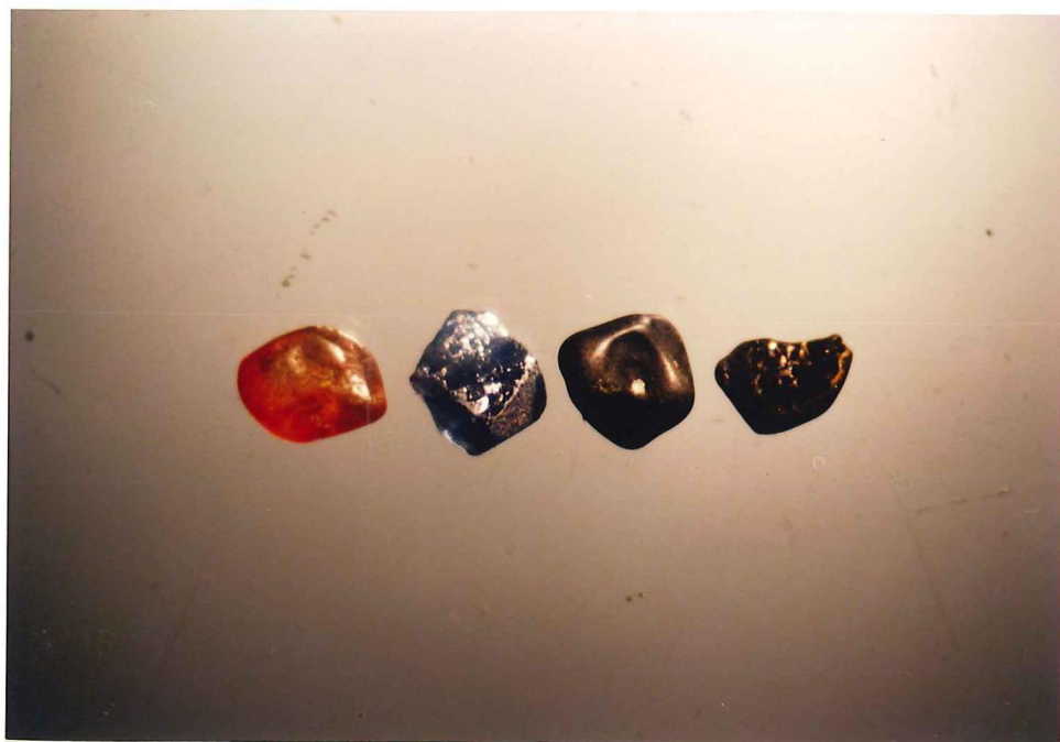
Plate 4.3 The zircospilic suite of heavy minerals. From left to right, the minerals are zircon, corundum, spinel and ilmenite. Mutual Mine. X 6.5.
