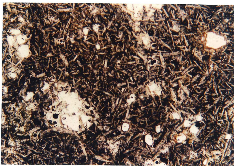
Plate 6.4 Photomicrograph of a bauxitic nodule showing basaltic texture from the overburden of the Pioneer Tin Mine. Plane polarized light. X25.
