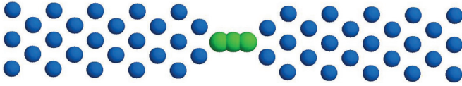
FIG. 2. (Color online) Schematic diagram of a molecular device Al-C 3 -Al. The device consists of a three carbon atoms chain coupled to the perfect aluminium atomic electrodes which extends to the reservoirs at \pm\infty , where the current is collected.
