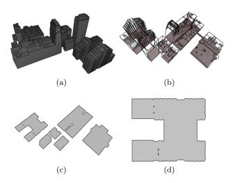
Fig. 3 Extracting the footprints of the buildings. (a) Group of buildings in down town Oklahoma. (b) Footprints and the buildings. (c) Only the footprints. (d) Detail of the footprint. The ground plan is composed for an outer boundary and four hole boundaries.
