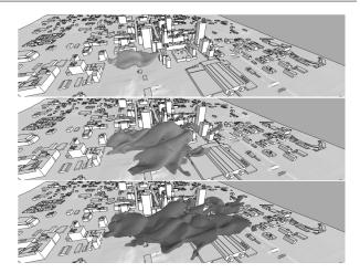
**Fig. 7** A cloud is depicted at 3 different time instances in the integrated Oklahoma City model. The cloud is transported and diffused by the effects of the wind and turbulence. Clouds at 100 (top), 250 (mid) and 500 seconds (bottom) from the beginning of the release.
