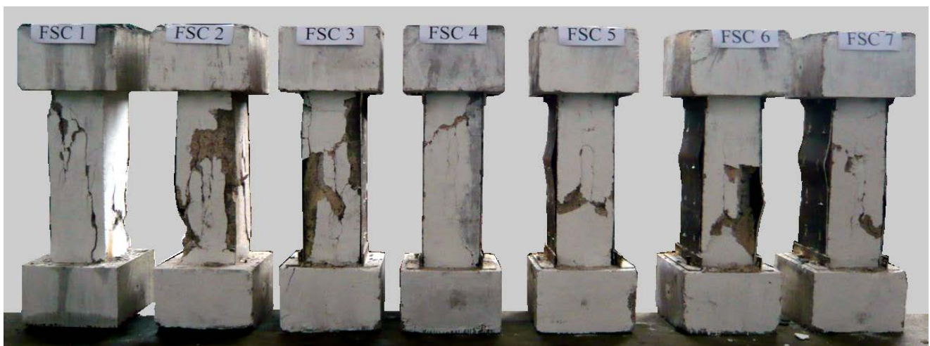
Fig. 11. Crack patterns and failure mode
