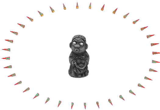
Fig. 1 Multiview stereo object reconstruction from a turntable image sequence. A sequence of images are taken from different points of view.
