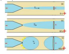
Schematics 1 A w/w jet breaks up in an electrohydrodynamic chopping approach. A viscous w/w jet (a,b) expands after electrical charging at 60 volts and (c) breaks up into droplets at 500 volts. The jet diameter increases ( $d_1 < d_2 < d_3$ ) with the applied voltage, while the jet velocity decreases ( $u_1 > u_2 > u_3$ ) accordingly.
