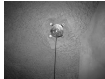
(c) Pressure cell installation
