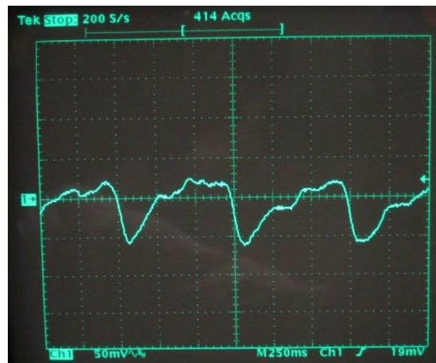
FIGURE 12. The pulse signal obtained by the infrared LED.
