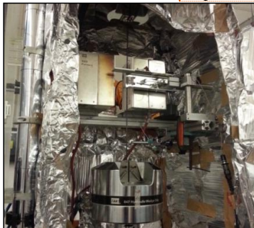
(a) MTS 810 Material Testing System
