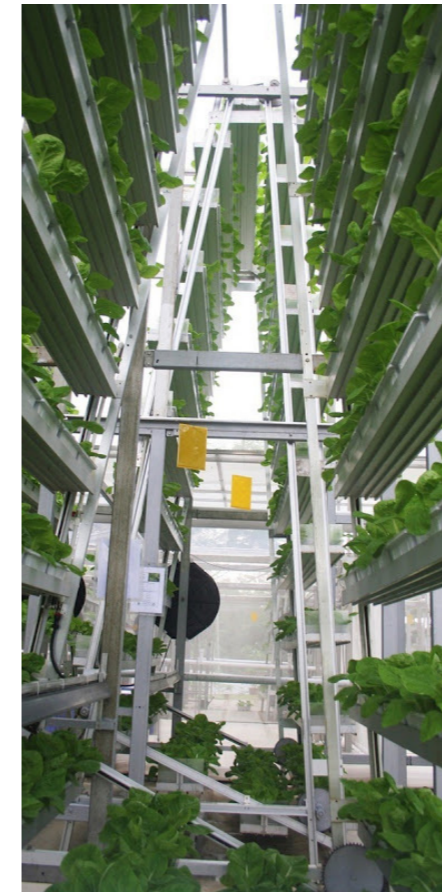
Jack Ng's vertical farm in Singapore uses a rotating structure to gain enough sunlight to grow salad vegetables (Photo: Amusing Planet)
