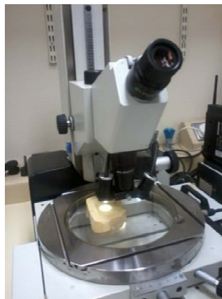
Figure 5b. Stone teeth model and the stent were loaded on the toolmaker's microscope for physically measuring the coordinates with reference to the origin O on the stent.
