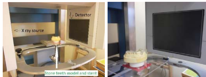
Figure 2b. The stone teeth model and the stent were loaded in the CBCT. The x-ray source and the detector moves simultaneously in one rotation during the imaging acquisition.
