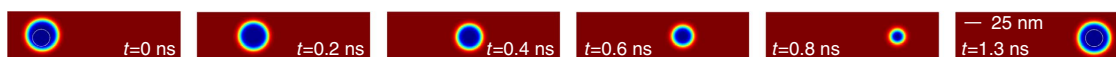
Figure 4 | Current-induced motion of a DS in a nanowire without DMI. A DS can be transported coherently between NCs along a nanowire without DMI, illustrating its quasiparticle nature. Initially, the skyrmion is nucleated and pinned at the left NC with a diameter of 25 nm. After switching off the spin transfer torque, the DS is released, continues to precess, and is transported coherently by an in-plane current to a second NC at a distance of 150 nm where it is trapped again and restored to its original size. Here the in-plane current density is 1.8 \times 10^9 \text{ A cm}^{-2} and the damping constant is set to \alpha = 0.05 with sample dimensions of 250 \text{ nm} \times 75 \text{ nm} \times 1 \text{ nm} . Here \beta = \alpha is chosen but very similar results are obtained for \beta \leq \alpha similar to the case of DMI stabilized skyrmions 14 . The white circles indicate the NCs. The red and blue colour indicate up and down magnetization, respectively.
