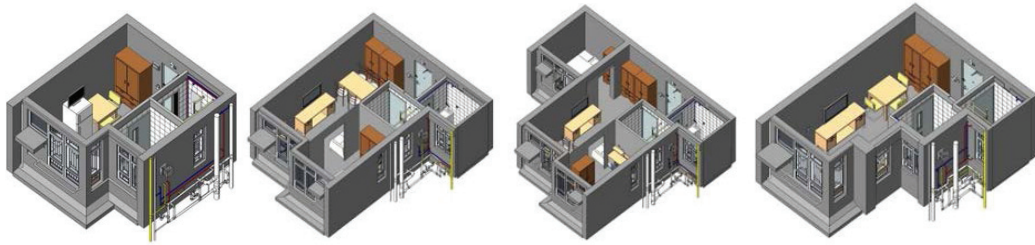
Fig. 2. From left to right (a) 1-2 person flat unit module; (b) 1-bedroom flat unit module; (c) 2-3 person flat unit module; (d) 2-bedroom flat unit module. Source: [20]
