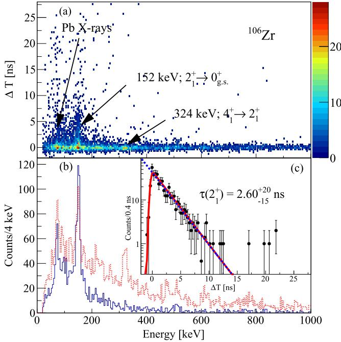
**Fig. 2.** (Colour online.) (a) Energy-time-difference matrix observed in coincidence with  $\beta^-$  detected within 0.3 s of an  $^{106}\text{Y}$  implantation. (b) The  $\gamma$ -ray energy spectrum of the delayed (solid blue) and prompt (dashed red) components of the matrix. (c) Background subtracted time difference spectrum for the  $2_1^+ \rightarrow 0_{\text{g.s.}}^+$  transition. (See text for details of the fits.)
