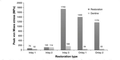
**Fig. 4** Peak von Mises stress values in the dentine and restorations for the five models subjected to oblique occlusal loadings of  $300 \, \text{N}$
