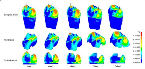
**Fig. 6** Von Mises stress patterns for the five models subjected to oblique occlusal loadings of 300 N; *arrows* indicate the locations of peak von Mises
