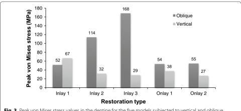
$\textbf{Fig. 3} \ \ \text{Peak von Mises stress values in the dentine for the five models subjected to vertical and oblique occlusal loadings of 300 \, \text{N}$
