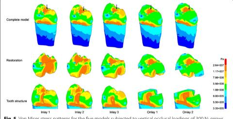
**Fig. 5** Von Mises stress patterns for the five models subjected to vertical occlusal loadings of 300 N; *arrows* indicate the locations of peak von Mises
