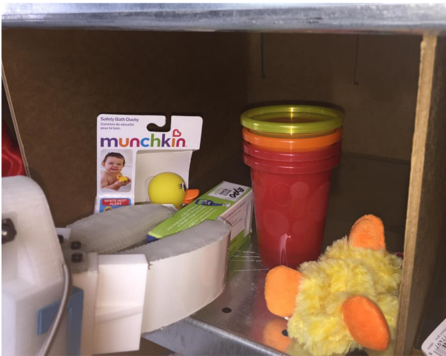
Fig. 7. Grasping one target object from a cluttered bin.
