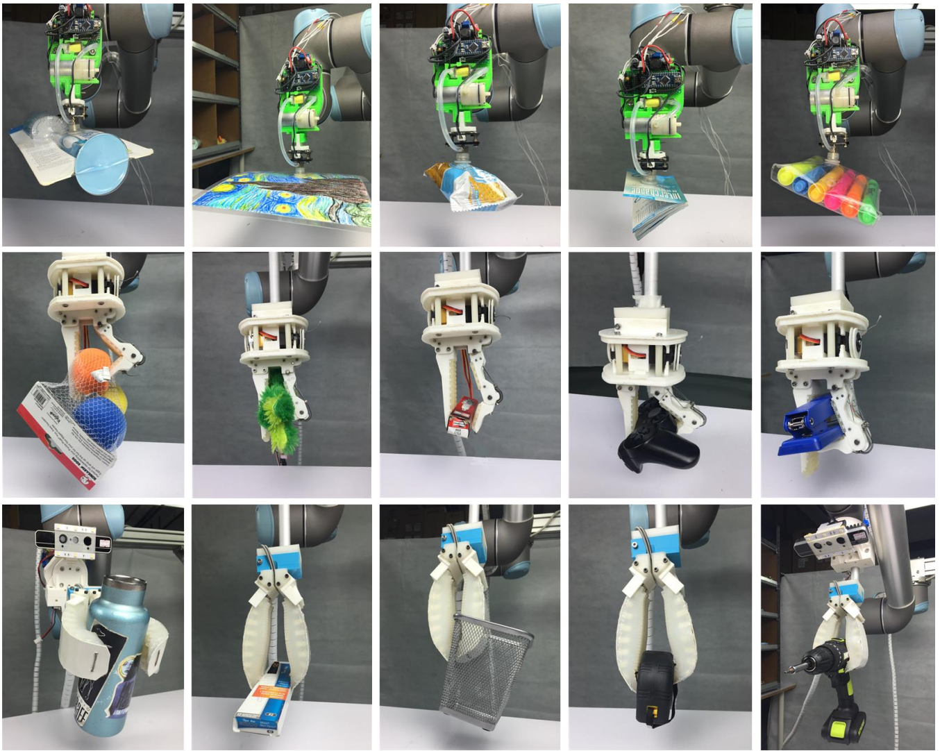
Fig. 9. Representative objects grasped by our three grippers.
