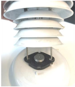
(a) An iButton housed in a solar radiation shield.
