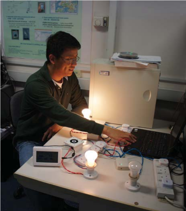
Figure 3-10 Testing the controllers and Control Logic for Smart Grid by Dr. Guanghua Yang
