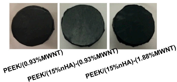
Figure 16. Photographs of Alizarin Red stained PEEK/(0.93% MWNT), PEEK/(15% nHA)-(0.93% MWNT) and PEEK/(15% nHA)-(1.88% MWNT) nanocomposites without cell exposure.
