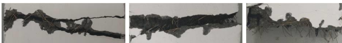
Figure 18. Bridging effect of the steel fibres at the cracks.
