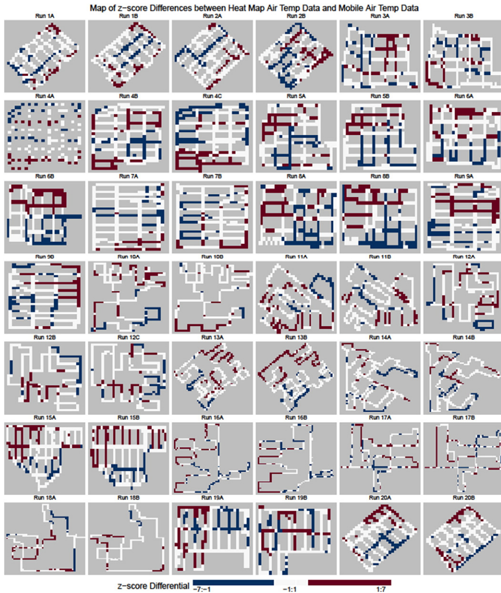
Fig. 5. Differences in the z-scores between the Greater Vancouver heat map (GVHM) and mobile air temperatures for all 42 runs. When interpreting, a positive z-score differential means that GVHM z-scores were higher than the mobile air temperature z-scores, suggesting that the GVHM overestimated air temperature. A negative differential suggests the GVHM underestimated air temperature.
