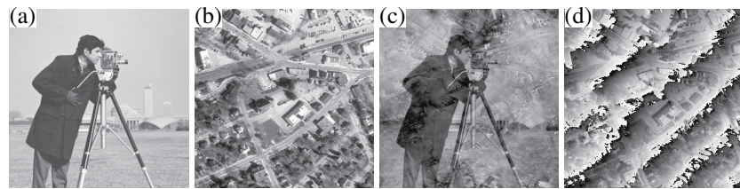
Fig. 4. A simulated reconstruction with a global shift in the FPM. Amplitude (a) and phase (b) profiles of the object and the reconstructed amplitude (c) and phase (d) profiles with a global shift.
