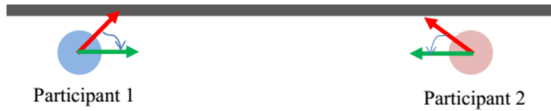
Fig. 4. Decision on wall-following direction for a participant who has just seen the wall. The red arrow represents the walking direction of the participant who has just seen the wall, and the green arrow represents his/her wall-following direction.
