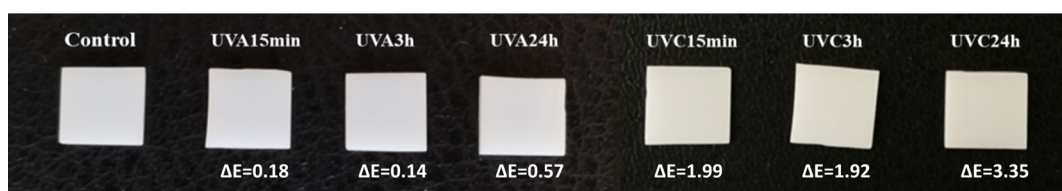
Figure 1. Zirconia samples irradiated with UV-A or UV-C with respect to different times (15 min, 3 and 24 h). NB: UV-C irradiation caused color changes in the samples. SEM images of surface morphology and EDX analysis.
