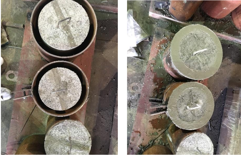
Figure 5. Casting of 2-Layer Specimens
