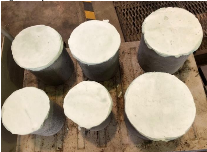
Figure 9. Specimens Covered with Dental Stone
