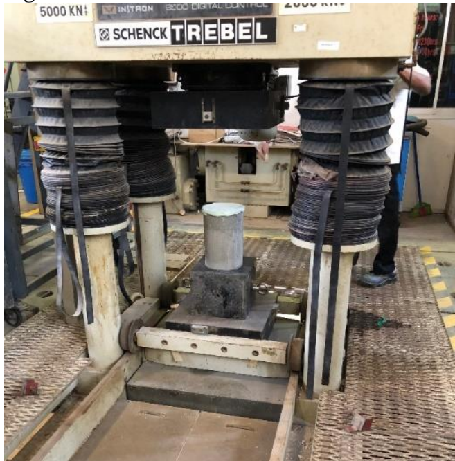
Figure 10. Steel Cube Base
