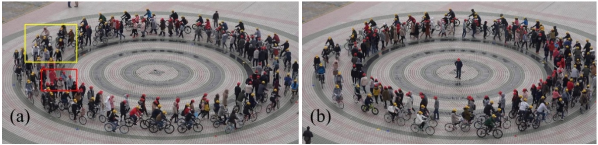
Fig. 7. Snapshots of 80 pedestrians + 80 cyclists experiment. (a) Unidirectional flow, (b) bidirectional flow.
